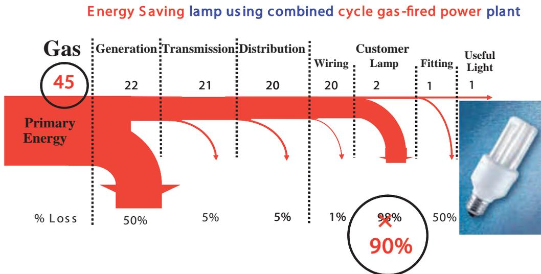
For a given light output, compact fluorescent lamps use between one-fifth and one-third of the power of equivalent incandescent lamps.
